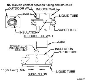
Fig. 1 - Connecting Tube Installation
